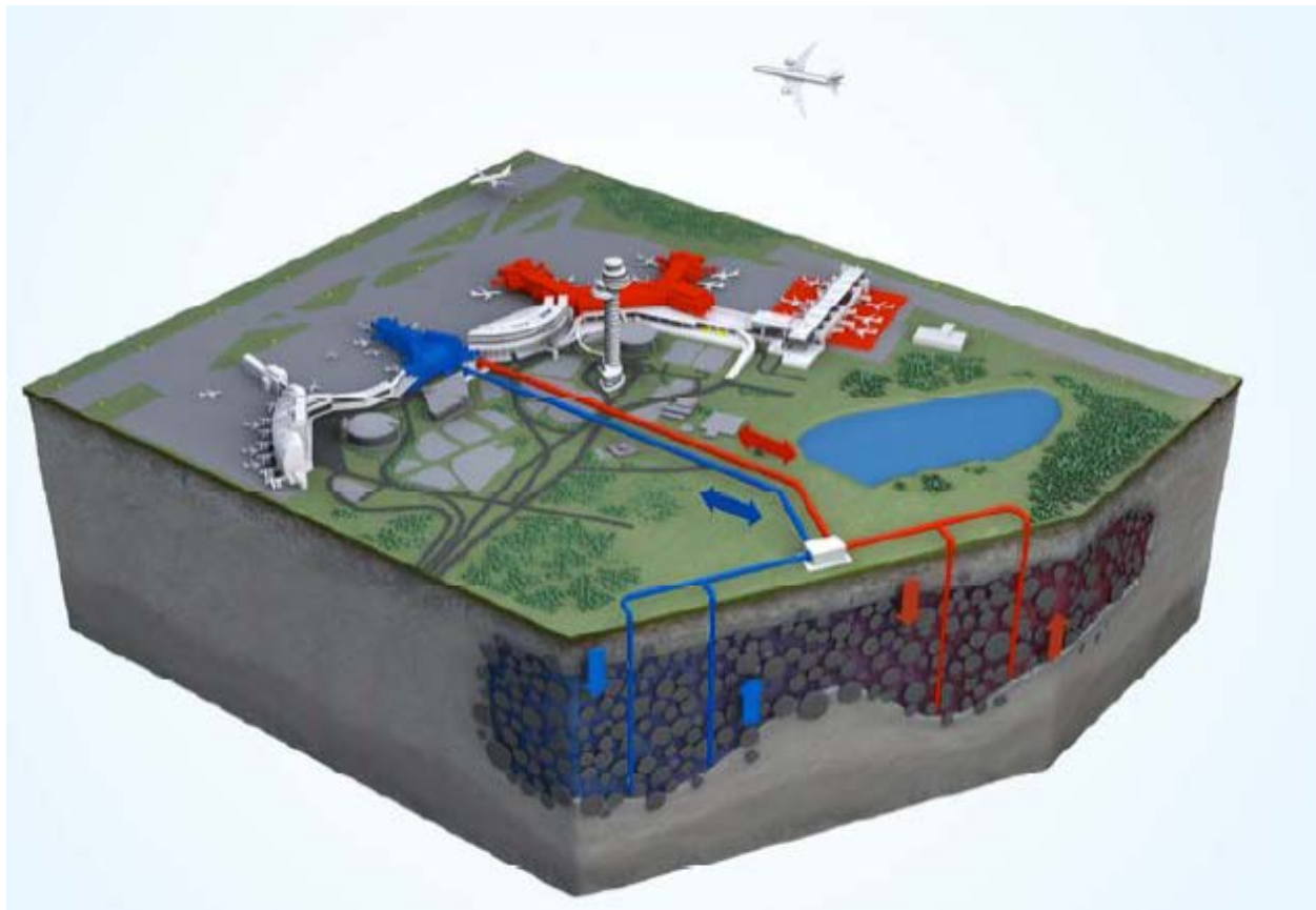
Figure 3. Schematic of ATES heats the airport terminal and the aircraft parking stands (Wigstrand 2010)
